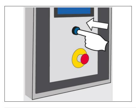
• Touch the **Reset** button. All components return to their **Home** position. When **Ready** appears on the HMI, the case former is ready for operation.
