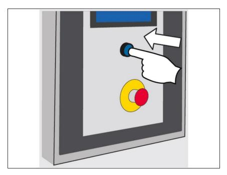
Touch the Reset button. All components return to their Home position. When Ready appears on the HMI, the tray former is ready for operation.
