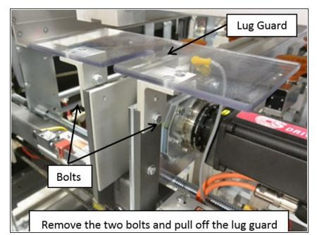
• Using a <sup>1</sup>/<sub>2</sub>" wrench, remove the two bolts that secure the lug guard and pull the lug guard off the machine.
